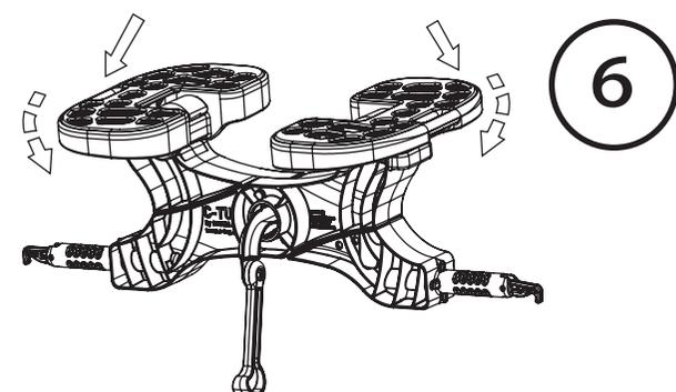
Continue to swivel the hull pad until it is flat. The hull pads will pivot to fit your kayak hull.
