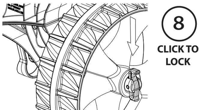
Push down on axle pin till it clicks into the lock position.
