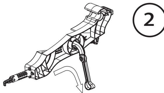
Pull kickstand completely through and ensure the pins in the kick stand base insert into the indentions on the inside of the Crossbeam.
