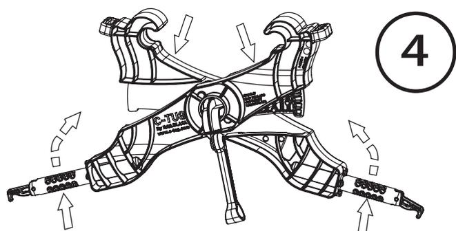
Compress both sides of the crossbeam and you should feel a click as the cross beam pins fit into the opposite side.
