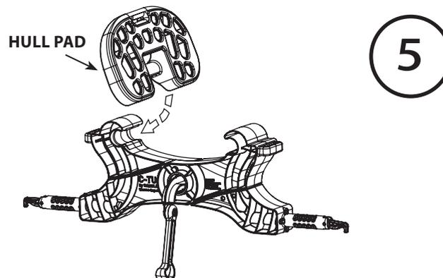
Swivel the hull pad into the hook.
