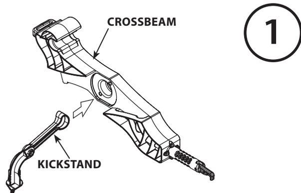
Slip the bottom of the kickstand into the inside of one of the crossbeams.
